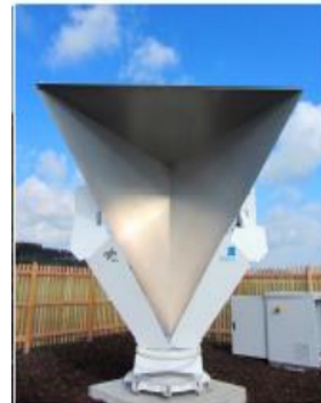
2.8 m DLR reflector in stowed position
