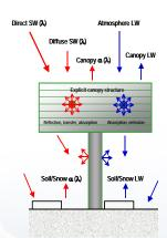
Gap probability-based successive orders of scattering approach that includes heterogeneity of stands and crown elements and the multiple scattering of radiation. Multi-canopy layers and multi-wavelength for solar radiation calculations. Separation of direct and diffuse radiation components. Outputs include surface (spectral) albedo, canopy (layer) and soll/snow surface solar radiation absorption, and longwave radiation balance. References: Wang et al. (2002a); Wang (2005); Wang et al. (2007).
